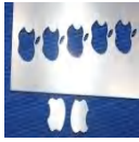
WT0.6mm stainless steel sheet cutting
